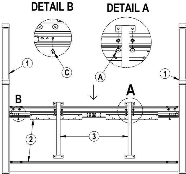
3) Insert the cross bar 3 between the side frames 2 and screw on with bolts A. (DETAIL A)
