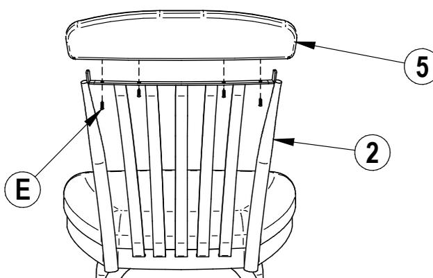
7) Insert the wooden backrest on the frame. Screw it on with E screws.
