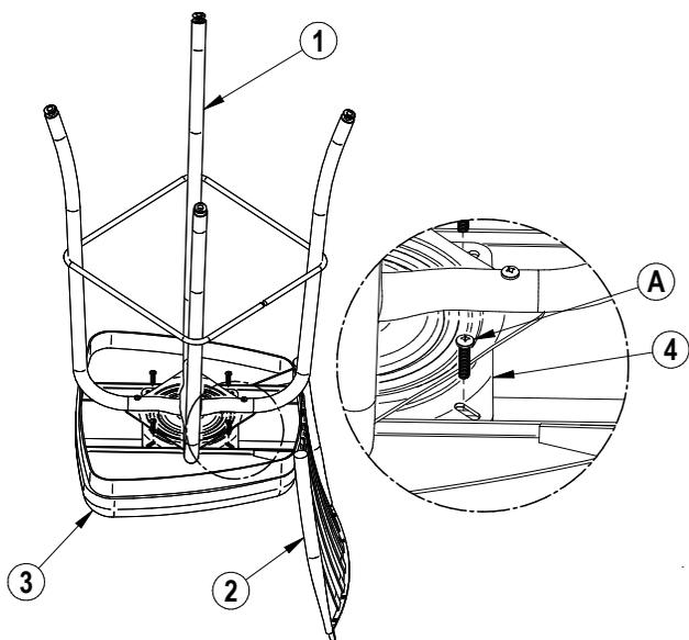
5) Place the 3 seat upside down on a stable surface, put the 2 welded backrest over it, then bolt-on lightly together the 4 swivel plate, the 2 welded backrest and the 3 seat with the B bolt.
