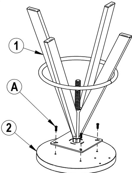
3) Place the seat **2** upside down on stable surface, put the stool base **1** over it, then bolt-on lightly together with the **A** bolts.
